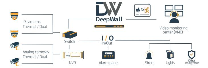
Deepwall's open philosophy allows it to work with existing installations, to operate on physical elements such as sirens and lights, and can be fully integrated into the software of central monitoring stations.
